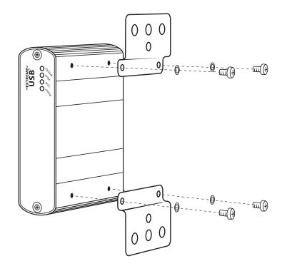
Once the bracket mounting is secured onto the extender, it is ready for mounting onto a surface. Please note you will need to provide your own screws to secure the extender using the available slots on each bracket.
