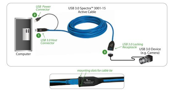
Conveniently secure your configuration by wrapping the included cable tie around the USB 3.0 receptacle's two mounting slots.
