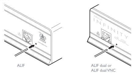
Use a straightened-out paper clip to press the reset button while powering on the unit
