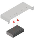
Install the two machine screws that are either provided with the product or need to be purchased separately.
