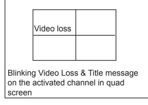
■ The warning message and the buzzer can be cleared by pushing Lock button (#2) for more than 4 seconds if the device is operated under Security lock On mode, or pushing any button on the front panel if the device is operated under Security lock OFF mode.
