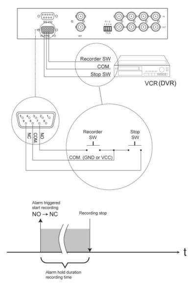
\*. If more than one sensor have been trigged, VCR will start to record after the last trigged event.
