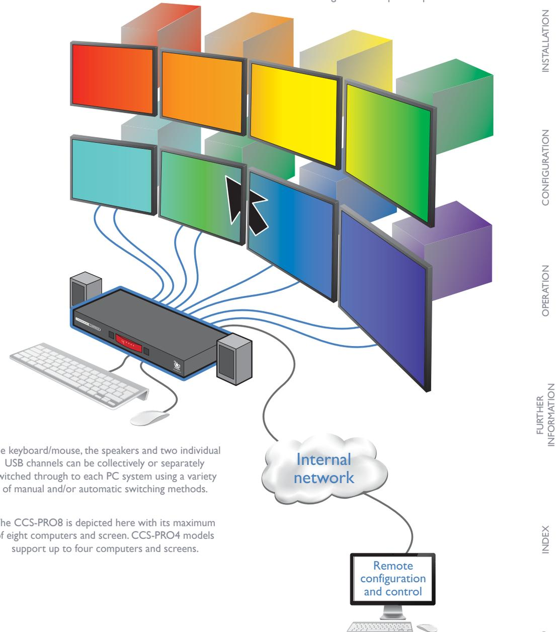
The keyboard/mouse, the speakers and two individual USB channels can be collectively or separately switched through to each PC system using a variety of manual and/or automatic switching methods.
