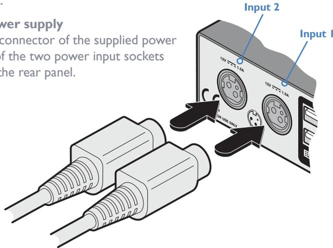
*Note: The outer sleeve of each power connector will retract slightly as it locks into place.*
